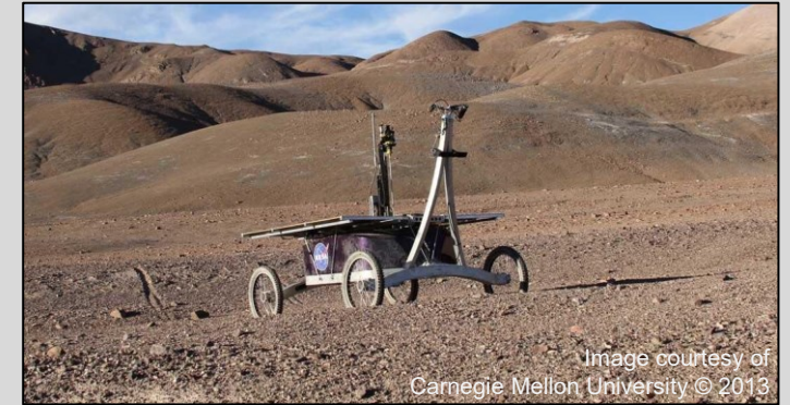
Autonomous rover traverse (26 km in 10 days) across the Atacama (CMU, 2015) TRL 5
