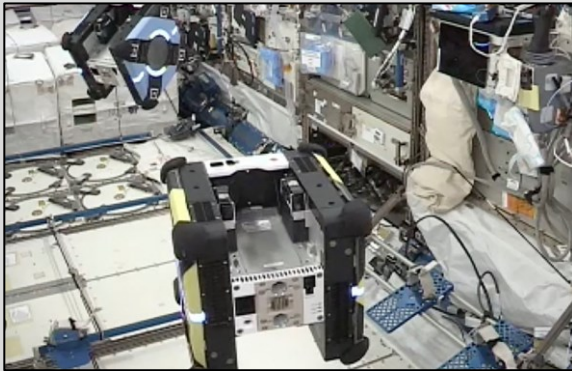
Astrobee, an operational ISS facility supporting IVA robotics R&D (ARC, 2019) TRL 7
