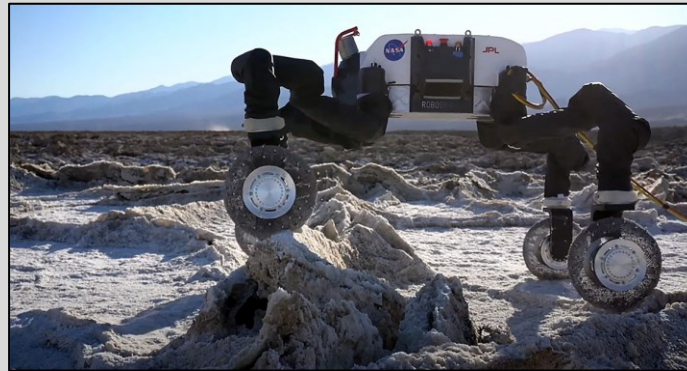
Traversing obstacles with 3x wheel radius with RoboSimian (JPL, 2020) TRL 5
