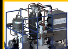
Water Capture, Cleanup, & PEM Electrolysis
